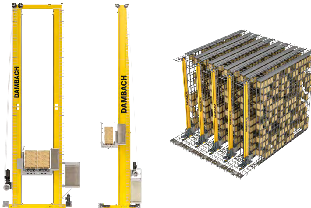
Figure 1: A single stacker crane (left) and a scheme of a warehouse with four aisles (right). The total mass of up to 40 tons in combination with heights of 30 meters lead to peak powers of several 100 kW (credit: DAMBACH GmbH & Co. KG).
