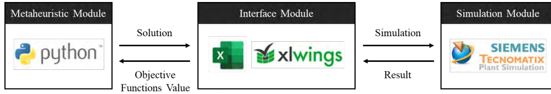
Figure 5: Interface procedure within the proposed system.
