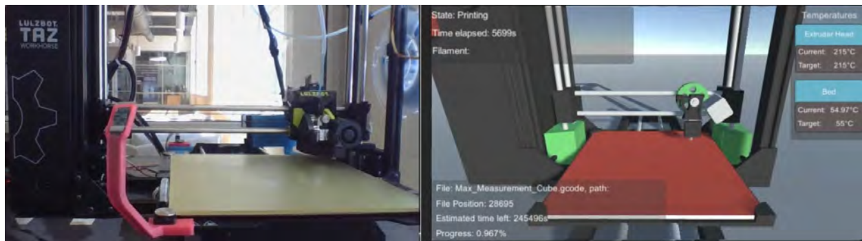
Figure 2: Left: Lulzbot TAZ Workhorse. Right: Process replication in the virtual domain captured from the Virtual Representation Component (Unity real-time development platform).
