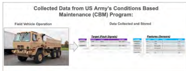
Figure 1: Description of Condition Based Maintenance dataset. Data from field vehicle operations, collected over several months from various vehicle types, are presented. This dataset includes time series of various fault signals, each with associated recording timestamps, as well as time series from multiple sensors also timestamped. Our analysis aims to utilize the sensor data as feature covariates to predict fault occurrences.
