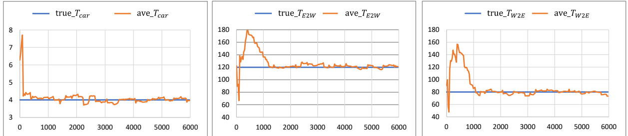
Figure 4: Online calibration of three parameters. The true T_{car} = 4.0s , T_{E2W} = 120s , T_{W2E} = 80s .
