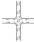
Figure 1: Typical four-lane road intersection.
