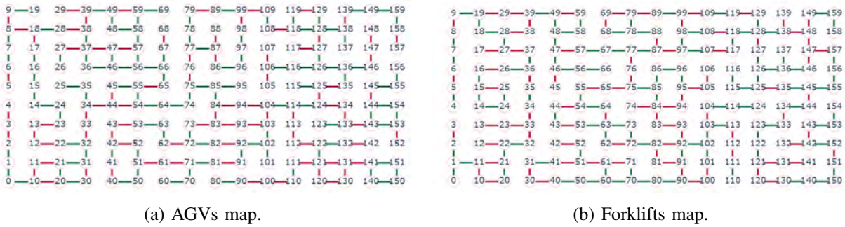
Figure 1: Example of warehouse layout with alternate traffic (red) and dual traffic (green) arcs for different vehicle classes.
