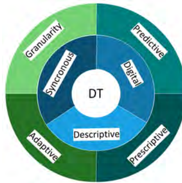
Figure 1: Basic features (inner circle) and advanced features (outer circle) of Digital Twins.
