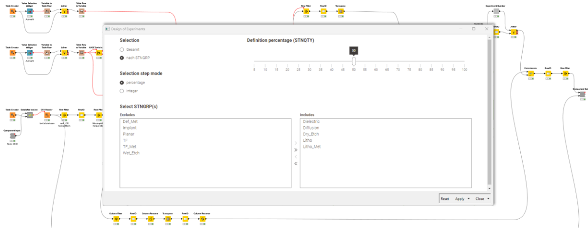
Figure 4: User interface and underlying process flow for the selection of factors for the design of experiment.
