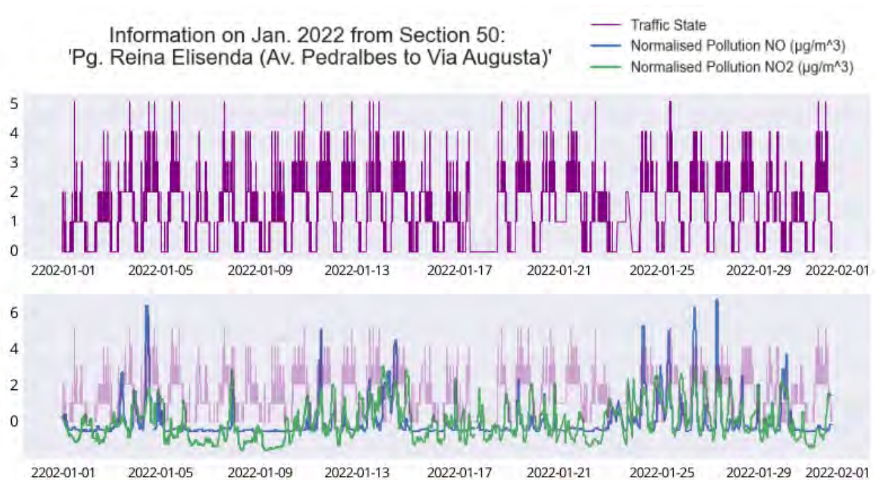
Figure 2: Comparison of two time series: original traffic density (top), generated normalised NO/NO 2 pollution (bottom).
