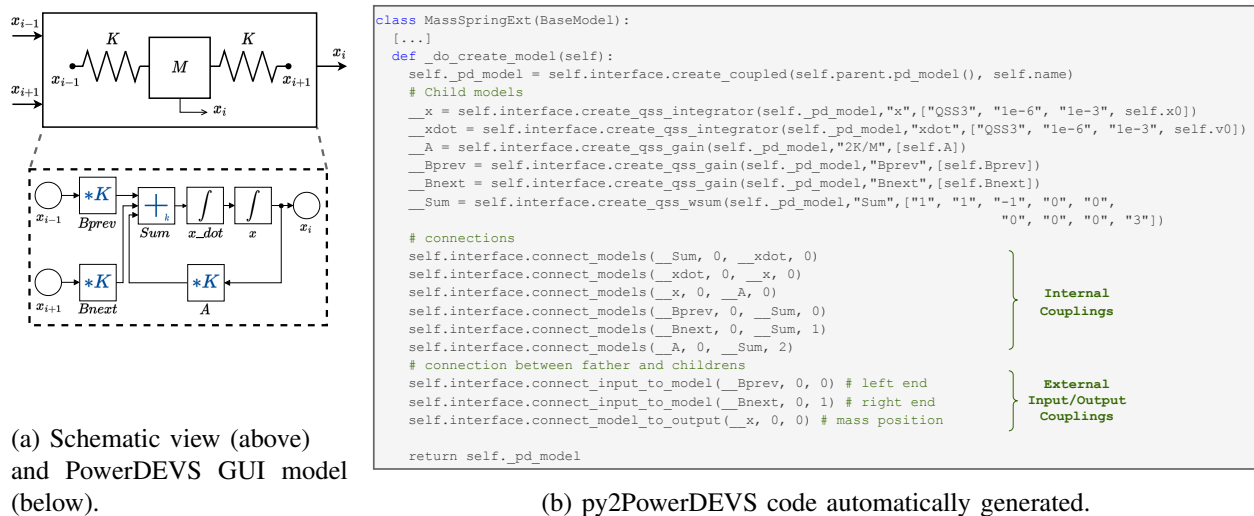
Figure 2: Mass-spring coupled model comprised of two integrators, three gains and a summation.
