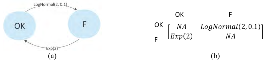
Figure 2: (a) A binary-repairable basic event with LogNormal failure probability distribution and the repair rate following an exponential distribution (b) Matrix version of the binary-repairable basic event in (a).
