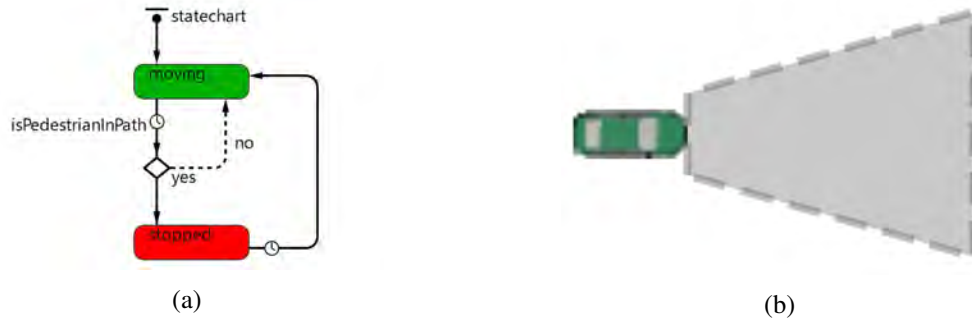
Figure 5: Pedestrian Detection. (a) State chart representing the logic for pedestrian detection, (b) CAV agent with front sensors to detect pedestrians.
