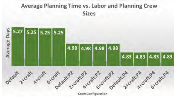
(a) Average planning time vs. crew & planning resource increases. N +craft means N extra agents for all craft types.
