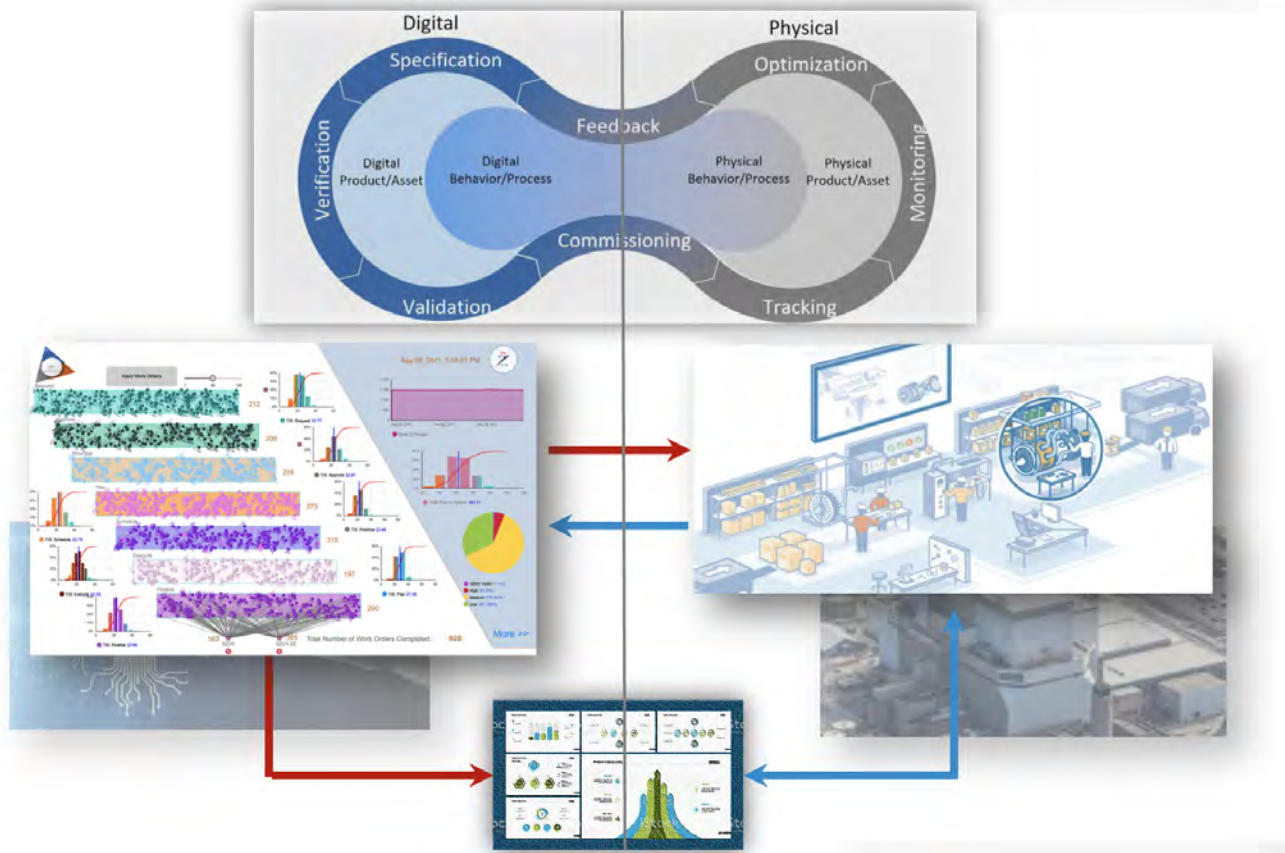
Figure 2: Illustration of MT process simulation model as an SDT: MT process and data are obtained to construct the simulation model, which guides the management to make operation decisions. Actual system operational data are collected to feed and update the simulation model. Such an iterative process continues to improve the overall SDT.
