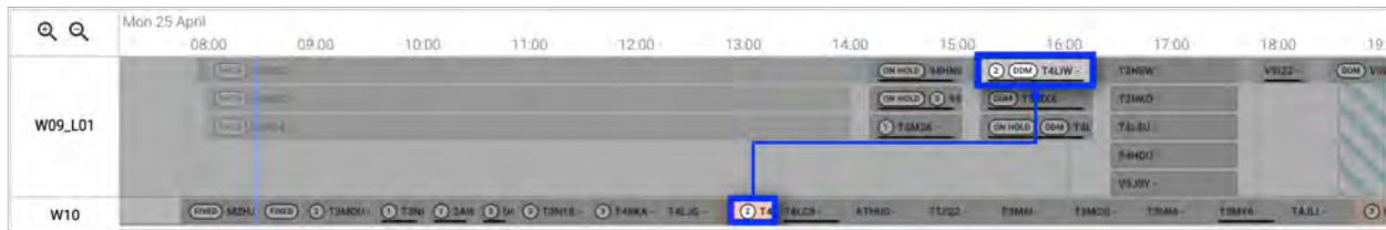
(b) With fab-wide scheduling: Wafer runs later allowing other wafers to go first.
