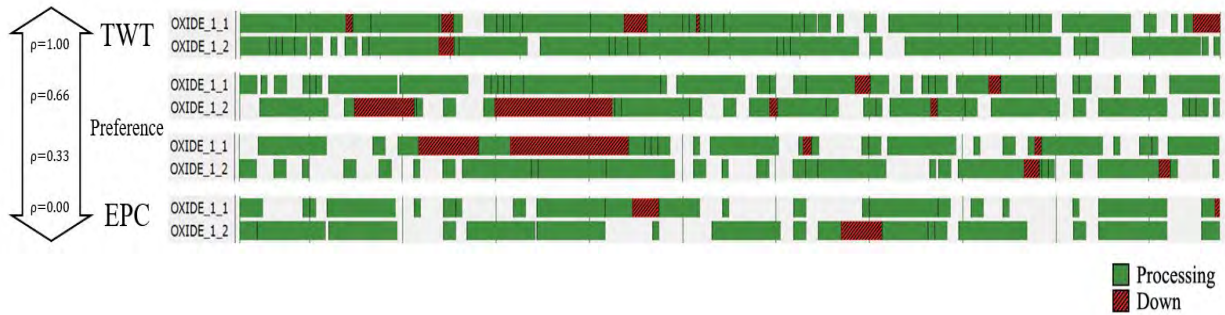
Figure 3: Visualization of the impact of preferences on machine utilization.
