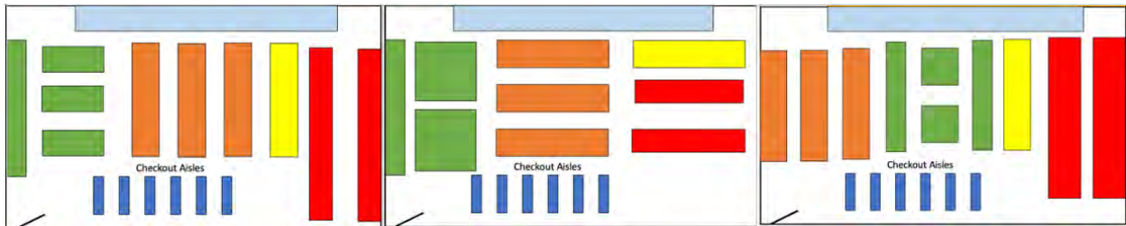
Figure 7: Three proposed layouts for a grocery store. The figure on the left, Layout 1, is the one used throughout the report. In Layout 2 in the center, many of the aisles are rotated to a horizontal orientation and the produce department shape slightly changes. On the right in Layout 3 the position of the grocery aisles switches with the produce section, and the produce section layout is altered.
