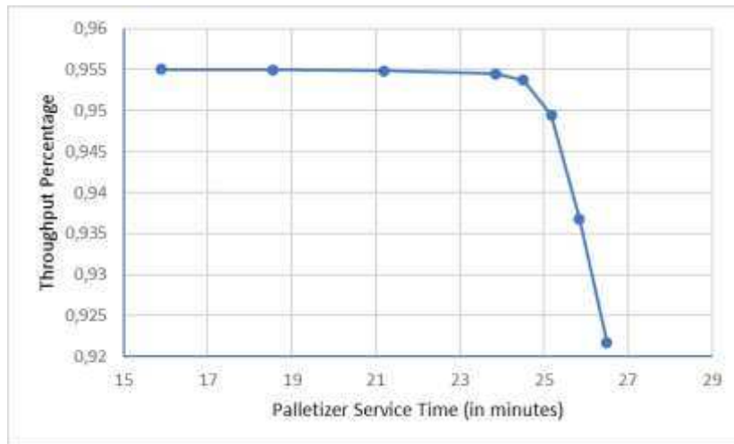
Figure 6. The Effect of Palletizer Speed Improvement on Throughput Percentage
