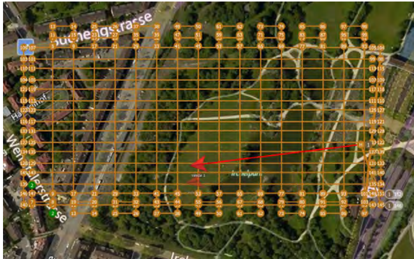
Figure 9: Two drones in survey mission area in Quad Ground Control (QGC).
