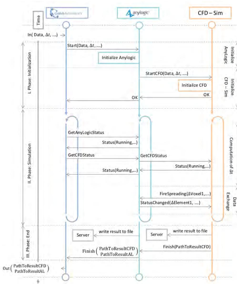
Figure 4: Principal scenario of a Co-Simulation Run.
