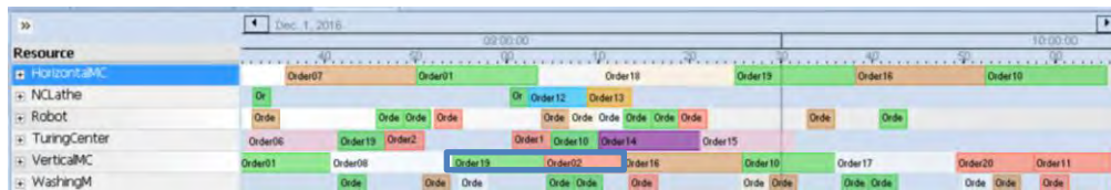
Figure 8: Rescheduling when a new order is inserted into the system.
