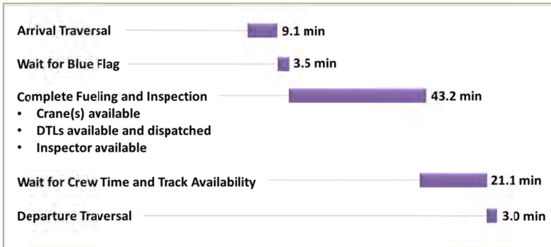
Figure 1: Processes completed for each train in the yard; times are representative of the current system.
