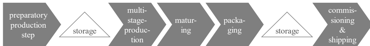
Figure 1: Simplified process overview of the production facility of the case study.
