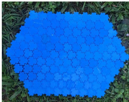
Figure 13. A 3D printed prototype for a stepping stone (Provided by S. Villanueva-Pérez et al.)
