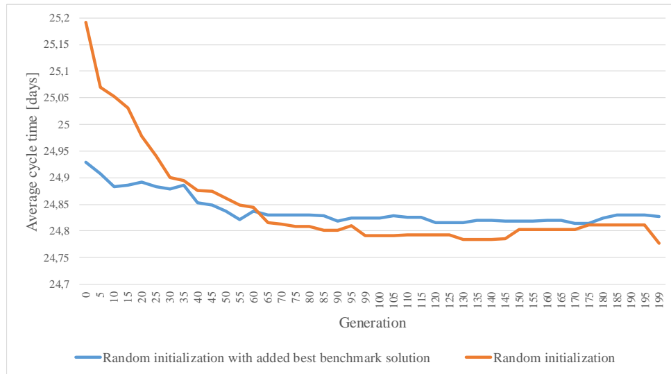
Figure 2: Convergence curve for optimizing the scenario “full” starting with random initial population vs. starting with random initial population and adding the best benchmark solution. Results are averaged over 10 optimization runs conducted for each method of setting the initial population.
