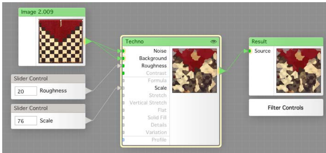
Figure 7: A data flow model that processes images using filter nodes. Program: Filterforge (Filterforge 2016).
