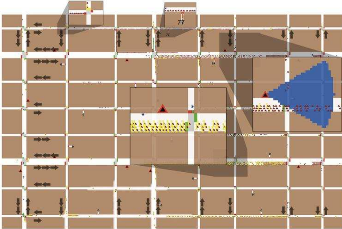
Figure 1: Simulation at 1800 ticks (15 minutes). The arrows denote the number of lanes in each direction. Black numbers show the contents of parking garages. Tiny colored numbers atop cars represent their AEGL states. A blue cone illustrates the visible region of a sample sign.
