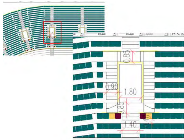
Figure 6: Dimension details of the stadium.
