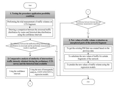
Figure 11. Data actualization procedure based on partially collected data and RM
