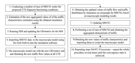
Figure 12. Procedure of macroscopic model application for MM data actualization
