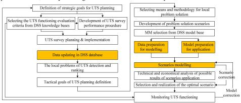
Figure 3. Model-driven DSS application in the frame of development plan for UTS
