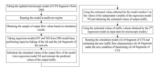
*Figure 14.* Procedure for data actualization for j-th MM based on the updated values of traffic of i-th MM (two intersections are located at different levels (road))
