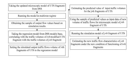
Figure 13. Data actualization procedure for j-th MM based on changed i-th MM data (two crossroads located at the same level (road))
