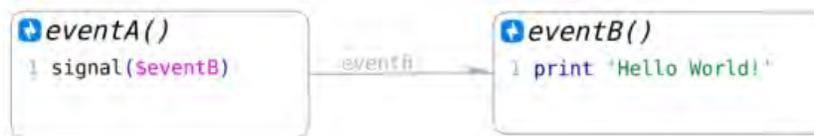
Figure 5: EventA sends a trigger signal to eventB containing no information. In this example, eventB responds by printing “Hello World!”, but the event could carry out any action required by the model.
