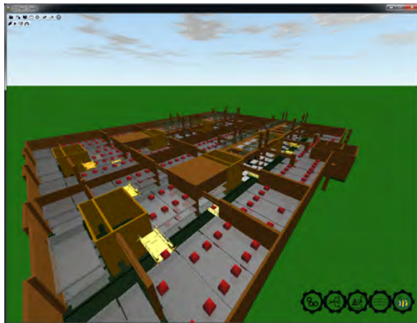
Figure 6: 3D visualization of the MHS in d 3 fact. An HM is shown in the foreground moving an object into a storage space.
