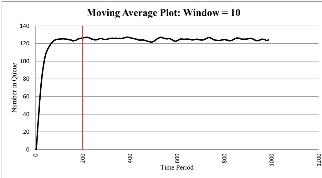
Figure 3: A plot of the moving average of the number of requests in the queue for the web server example, where the window length is set to be 10. The suggested warm up length is denoted by a vertical line.
