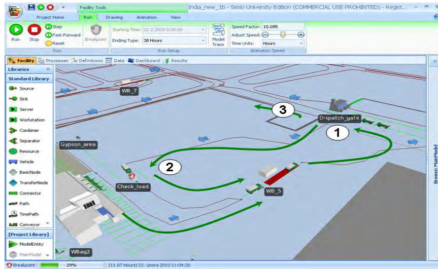
Figure 8: Rejection procedure for loaded trucks
