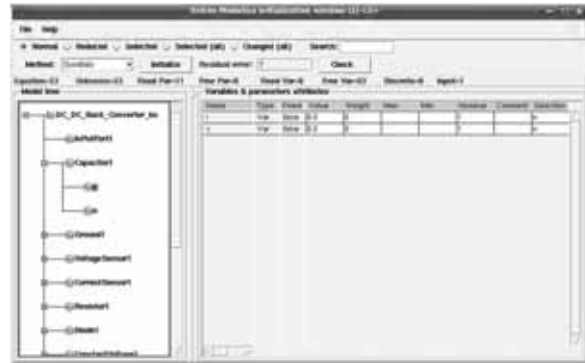
Figure 4. Screenshot of the initialization GUI in Scicos for the electrical circuit of figure 2.
