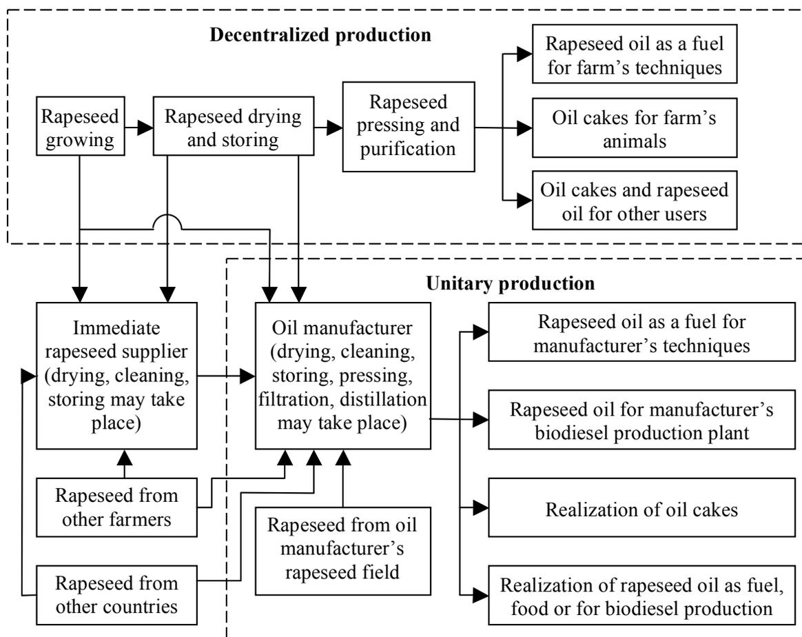
Figure 4. Rapeseed oil supply chain for decentralized and unitary production.
