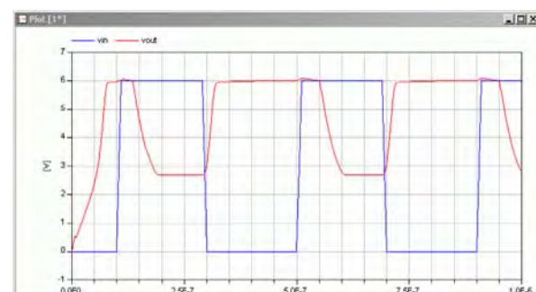
Fig. 12 Results of BondLib analog inverter simulation
