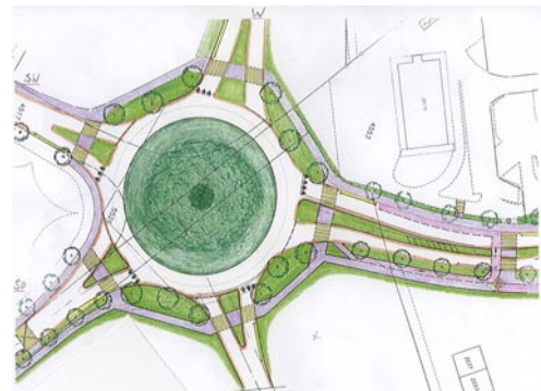
Figure 2: Single Tracked Roundabout with Multiple Pedestrian Crosswalks
