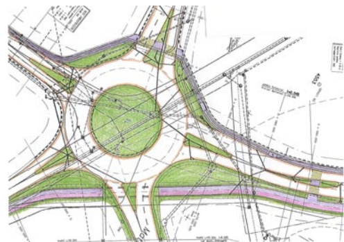
Figure 3: Double Tracked Roundabout with Special Tracks for Pedestrians and Bicycles
